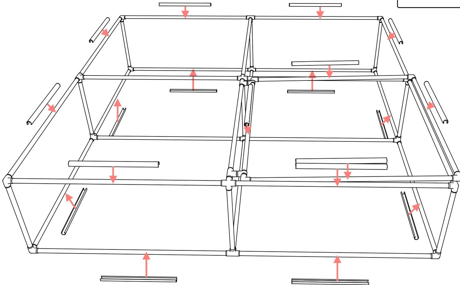
Use PipeClamps or zip ties to secure mesh netting or tarp(s) as needed. Allow access for the door to be opened by applying mesh/netting/tarps to the door separately.
