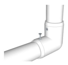
This method is not recommended for PVC pipe sizes 3/4" and under.
