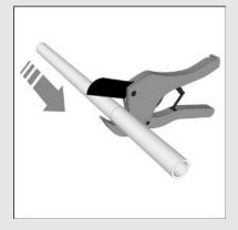
Grasp the handle with pressure until it the blade meets the mark, then release the handle and repeat to use the ratcheting action.
