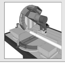
Pull the switch trigger and slowly bring the miter saw arm down into and through the pipe.
