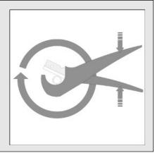
Once you have made one pass around the entire pipe, apply additional pressure and repeat the rotations around the pipe until it is cut through completely.
