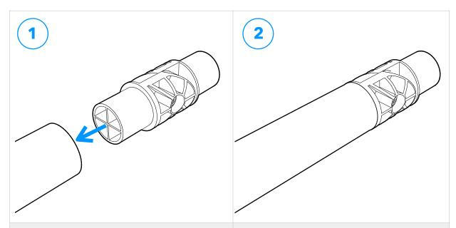
Line up and insert one end of the adjustable elbow inside a Schedule 40 PVC pipe segment. PVC cement or screws should be used to connect the internal adjustable elbow.
