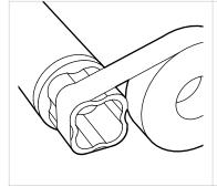
Use PVC cement to connect the internal-fit fitting into the pipe for a permanent connection.
