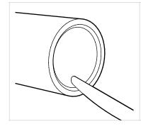
Run a kitchen knife or blunt object around the edge of the inner diameter of the pipe to taper it. This will allow easier insertion of the internal-fit item into the pipe.
