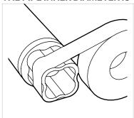
Use PVC cement to connect the internal-fit fitting into the pipe for a permanent connection.
