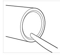
Run a kitchen knife or blunt object around the edge of the inner diameter of the pipe to taper it. This will allow easier insertion of the internal-fit item into the pipe.
