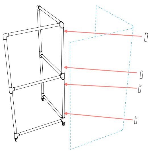
• Pull the plastic sheeting and apply the remaining PipeClamps along the outer perimeter of the partition and snap them onto the PVC pipe segments.
