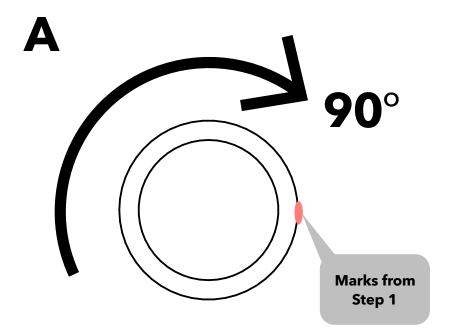
A. Rotate the same 48" pipe 90 degrees so that the previous marks are now on the side of the pipe.
