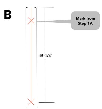
B. On the same side of the pipe, measure down 15-1/4" **from the top**, and make a mark.
