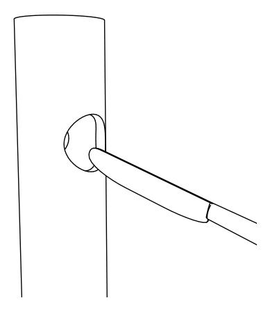
B. Use a butter knife or other blunt tool to remove 'burrs' from the cut pipe, by running it around the edges of the corners of each hole.
