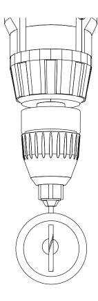
A. For each of the three marks you made, drill a pilot hole using a 1/4" drill bit **through both** sides for the pipe. Try to keep the drill bit at a perfect right angle to the opposite side of the pipe.
