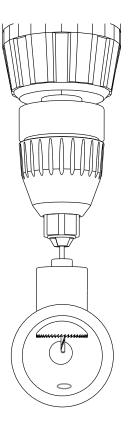
B. Once each pilot hole is finished, drill a 1-1/8" hole saw into each of the pilot holes, to cut out larger holes in the pipe. When one side of the pipe his done, flip the pipe over and do the other side (don't try to go through both sides with the hole saw).
