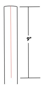
B. On the new side of the pipe, measure down 9" **from the top**, and make a mark.
